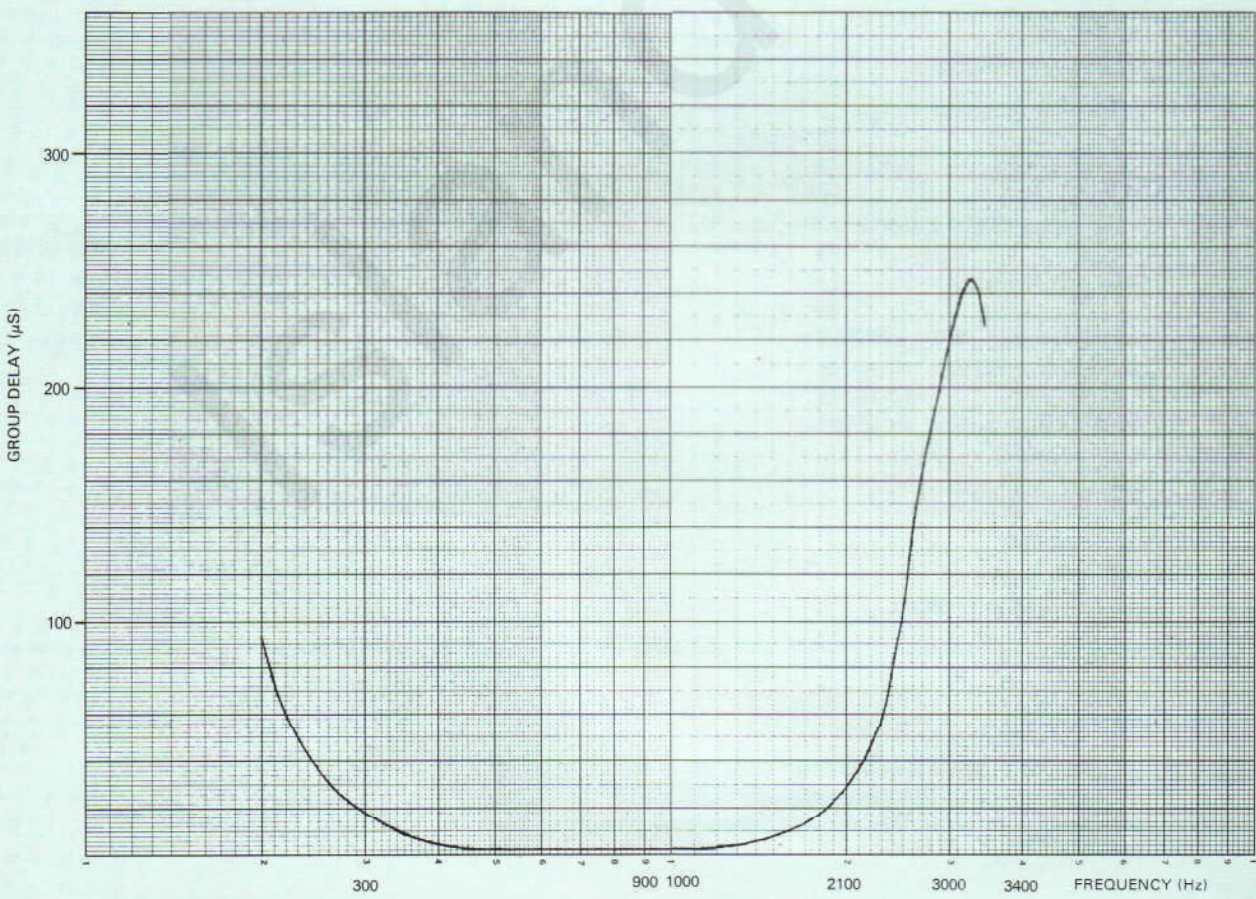
Fig. 5 FX306 Typical Group Delay Characteristics
